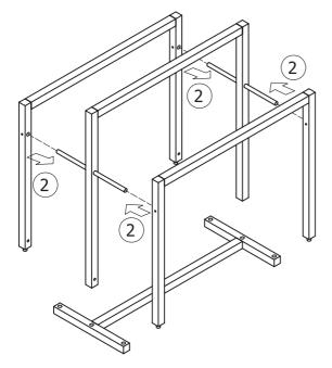
3. Rotate the pipes to reach position for wooden dowel to be fixed. Fix in the wooden dowel.
