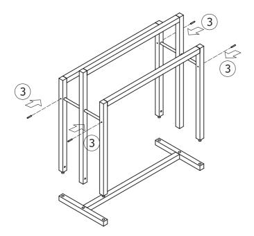
4. Adjust the position of the middle structure to be centered on the pipes. Place the assembled structure on the food and screw the six bolts with the six cross dowel on the structure.
