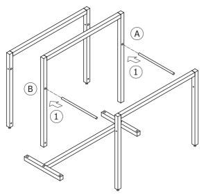
2. Position the side structures in order for the pipes to slide in teh holes of side structures.
